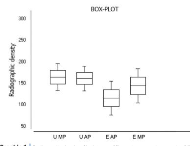
**Graphic 1** Radiographic density of both types of films using manual processing (MP) and automatic processing (AP).
