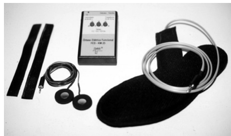
Figure 4 - Functional Electrical Orthosis - FES system with sensor pad
