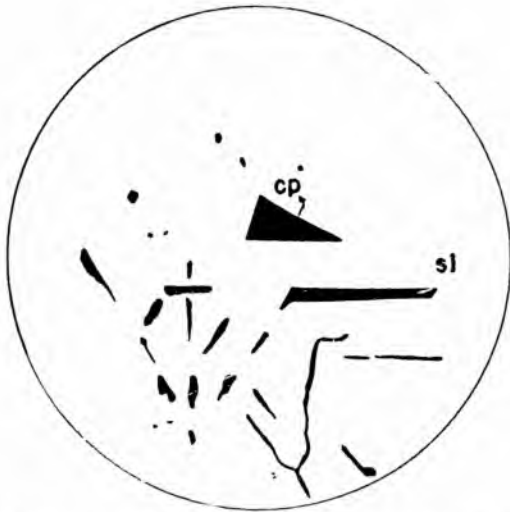
FIG. 13 — Different shapes of chalcopyrite inclusions following sphalerite cleavage planes. (Telluride 1018 — Harvard collection). Approximate magnification: 140 X.
