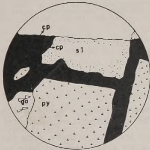
FIG. 1 — "Non-exsolved" and "exsolved" chalcopryrite. The first kind seems to be replacing both pyrite and sphalerite-chalcopryrite inclusions. (Telluride 1017 rite. Borders of sphalerite richer in — Harvard collection). Approximate magnification: 140 X.
