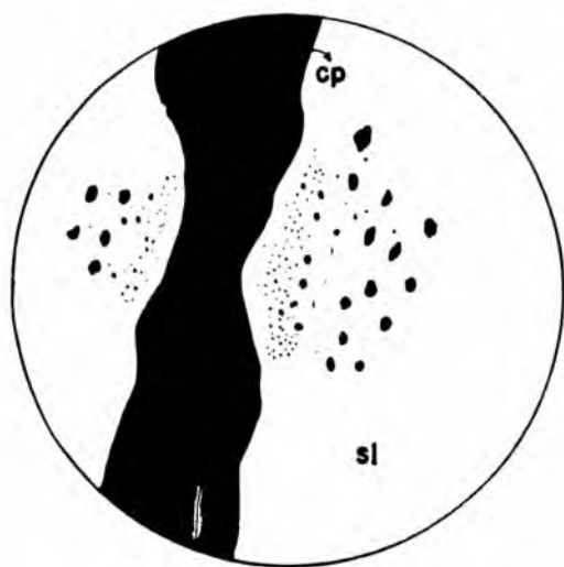
FIG. 9 — "Non-exsolved" and "exsolved" chalcopyrite. Zoning of sphalerite grains revealed by the different sizes of chalcopyrite inclusions. (Porcupine 66 — Harvard collection). Approximate magnification: 140 X.
