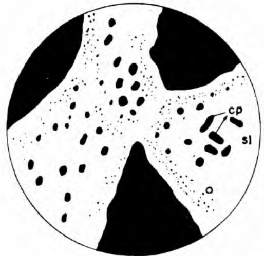
FIG. 26 — "Replacing" and "exsolved" chalcopyrite. Zoning of sphalerite grains revealed by variation of the chalcopyrite inclusions sizes. (Cananea 1085 — Harvard collection). Approximate magnification: 140 X.
