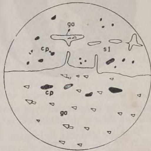
FIG. 2 — Galena is replacing selectively the sphalerite, but not attacking the chalcopryrite blebs. Galena is confined to sphalerite grain boundaries. (Ouray 1154 — Harvard collection). Approximate magnification: 140 X.
