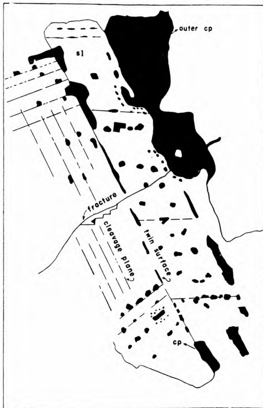
FIG. 4 — Different shapes of chalcopyrite inclusions, which are following cleavage and twinning planes of sphalerite. Outer chalcopyrite (replacing). (Cananea 1229 — Harvard collection). Approximate magnification: 140 X.
