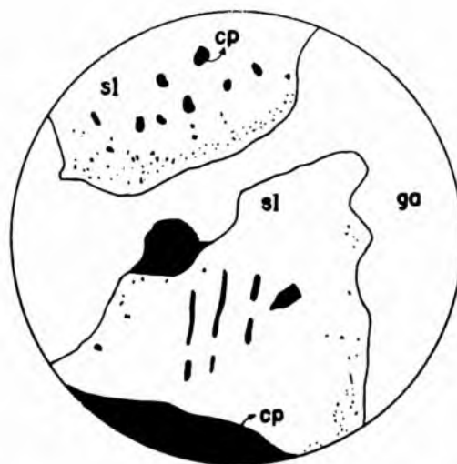
FIG. 10 — Large range of variability in the size of the chalcopyrite inclusions. (Silver Bell 1005 — Harvard collection). Approximate magnification: 140 X.
