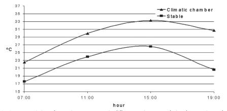
Figure 1 - Average variation of operative temperature in different environments during the experimental period
