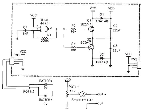
Figure 2 - Electronic diagram of the small iontophoresis device
