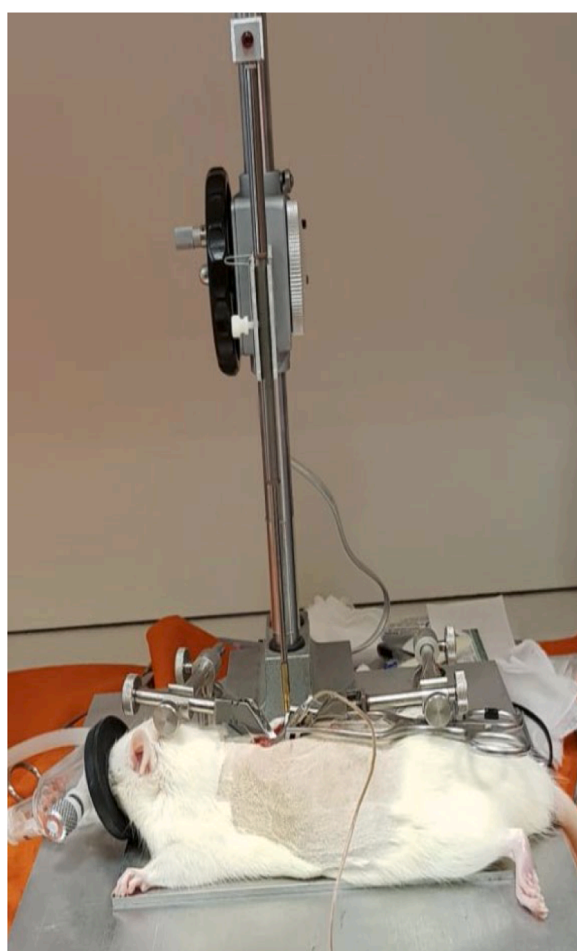
Fig. 2. Spinal impact using the NYU Impactor.
