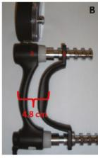
Figure 2. Detail of the standardized distance in the handle for hand grip: A - load cell; B - Jamar® dynamometer
