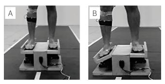
Figure 1. Inicial moment (A) and final (B) of the opening of the invertion platform at 30 degrees
