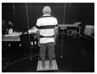
Figure 1. Acquisition of stabilometric data
