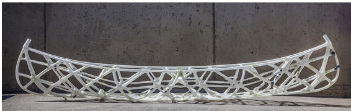
Figure 15: The 84 3D printed pieces assembled and ready for casting. Source: DBT, ETH Zürich, 2017
