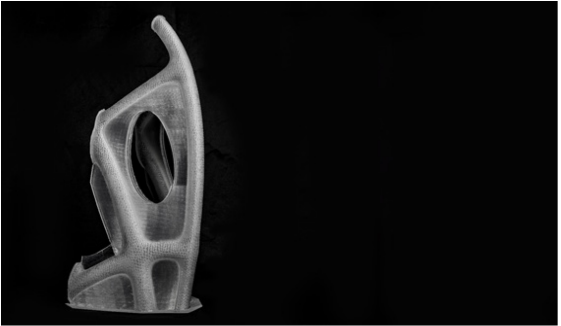
Figure 12: A 700-mm tall sample 3D printed part of the skelETHon formwork. In order to prevent quality issues for taller parts, a membrane-like auxiliary support structure is introduced.
