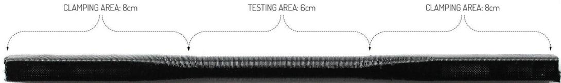
**Figure 7:** The scheme shows dimensions and geometry of the testing specimen
