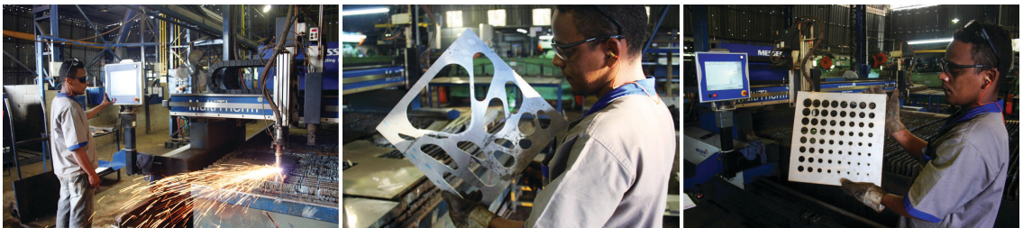
Figure 19. CNC plasma cutting process showing different designs.
