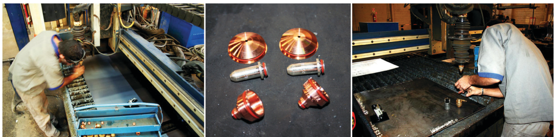
Figure 20. Changing torch consumable parts (photos by Wilson Barbosa).
