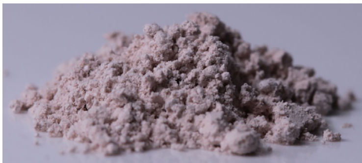
Figure 1- MnO-doped Biosilicate® (MnO_BioS) powder after agate milling in a planetary mill.
