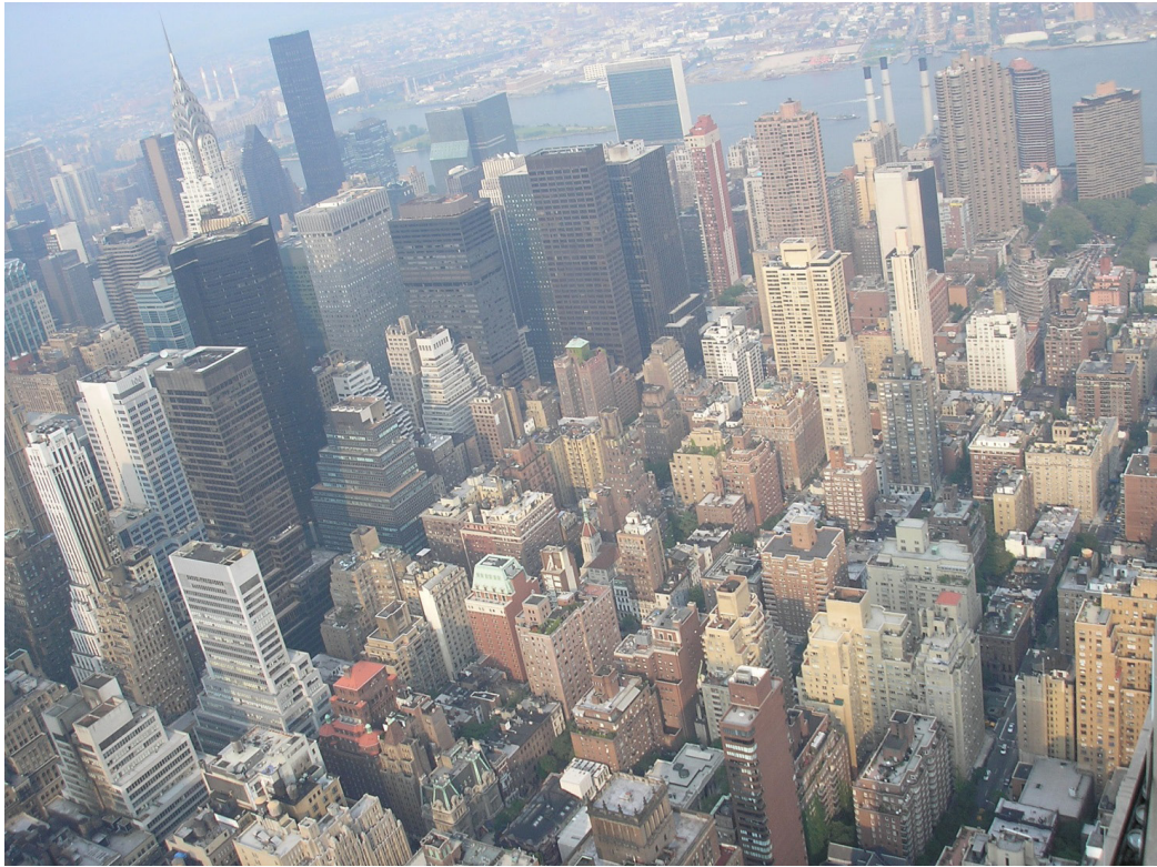
Figure 3 View from above of the Eastside of Manhattan with many staggered buildings, due to urban constraints from the 1916 Zoning Resolution. Photo: The author, 2013.
