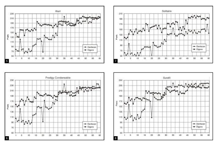
**GRAPHS 5, 6, 7 and 8** - Comparison between the values of optical density obtained by means of the DentScan Dent-View<sup>®</sup> and Digora<sup>®</sup> digital systems, for each of the four packable composite resins. Porto Alegre, 2002.
