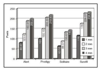
**GRAPH 3** - Mean values of optical density of each of the four packable composite resins, in the different analyzed thicknesses, using the DentScan DentView<sup>®</sup> digital system. Porto Alegre, 2002.
