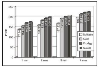
**GRAPH 2** - Mean values of optical density of each of the four packable composite resins, using the Digora<sup>®</sup> digital system. Porto Alegre, 2002.
