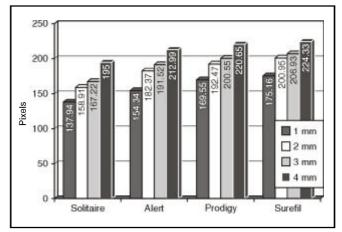
**GRAPH 4** - Mean values of optical density of each of the four packable composite resins, in the different analyzed thicknesses, using the Digora<sup>®</sup> digital system. Porto Alegre, 2002.
