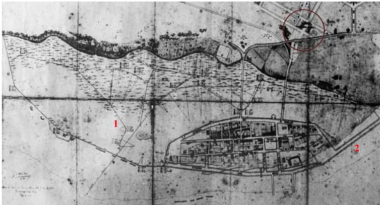
Figure 2 – Junta de Investigação do Ultramar [signature unreadable], extract of the “PLANTA GERAL COMPREHENDENDO/ Planta da nova povoação/ Projecto de esgôto do pantano/ Projecto de melhoramentos na povoação antiga e porto”, Lourenço Marques, 1878. The project for the improvement of the colonial settlement included the sanitation of the Maé marsh (1) and the expansion of the port to the downstream (2). The new hospital and the new parish church appeared under the plan of a “new town” in Alto da Maxaquene (indicated by the circle). Source: CEDH-FAPP.
