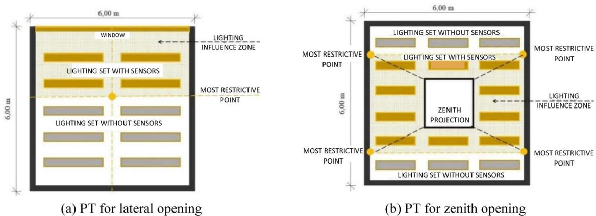
Figure 2 - Example of PT location for lateral and zenith opening
