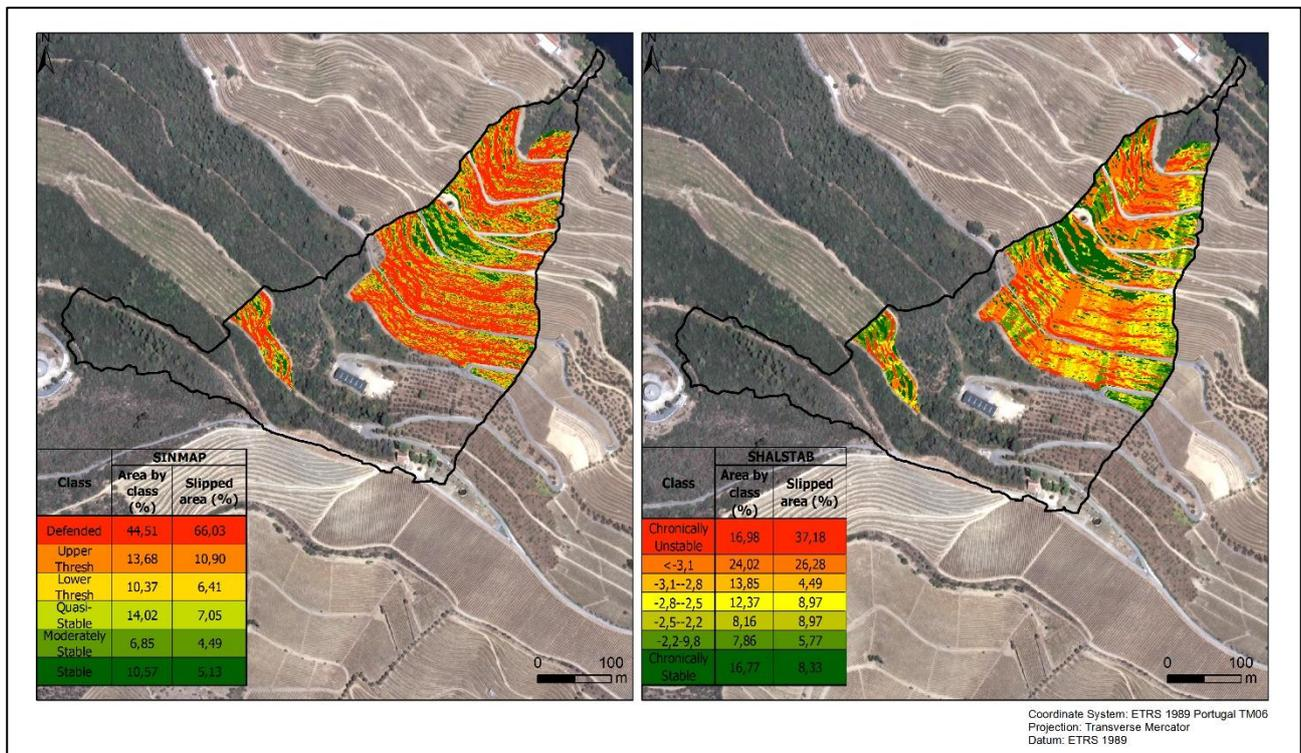
**Figure 2:** Susceptibility to landslide modelling with SINMAP and SHALSTB and contributing areas respectively.
