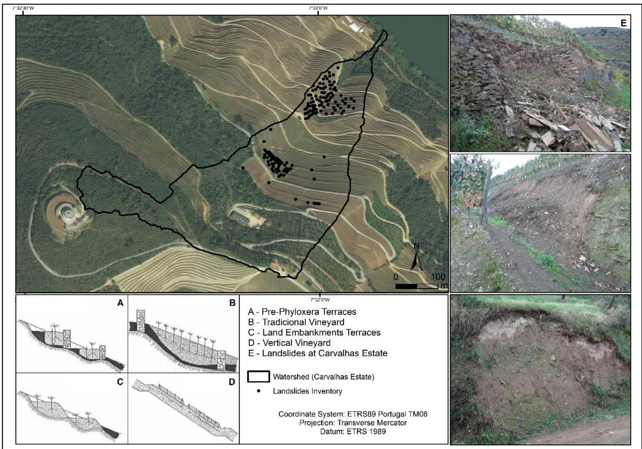
**Figure 2: Landslides inventory at Carvalhas Estate and Types of terraces in the Douro Valley.**
