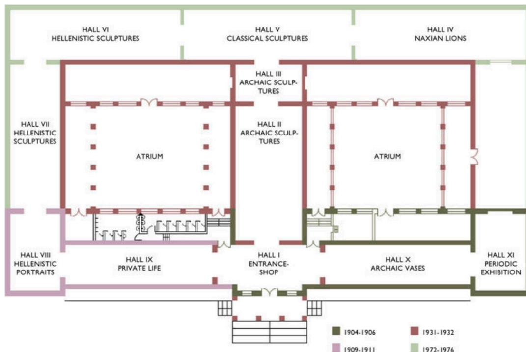
Fig. 4. Plan showing the construction stages of the Museum of Delos.
