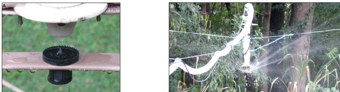
Figure 7 – Variable rate sprinkler operating in spraying conditions with smaller water droplets. A) utilized fixed deflector. B) visual aspect of the spray.
